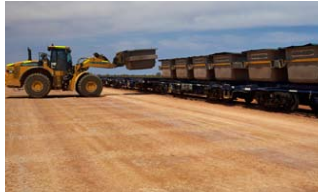
Loading kibbles onto a road train
