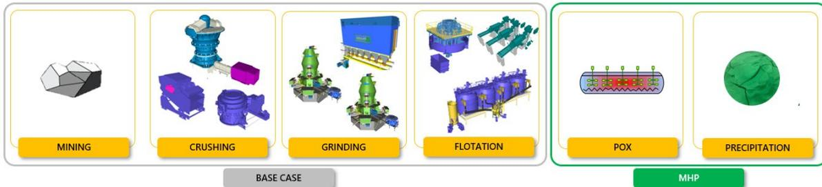
**Figure 1: WMP Flowsheet including additional MHP process**
